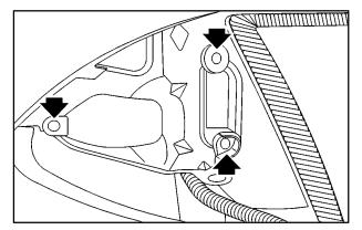
5. Align the outboard pin to the outboard tab in the bracket. Align the (two) inboard pins with the hole in the headlamp bracket.
